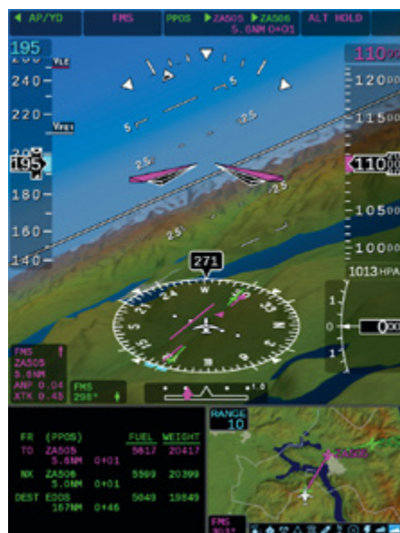
PFD with 360° HSI, Left Inset with Flight Plan Data, Right Inset with Map and SVS
