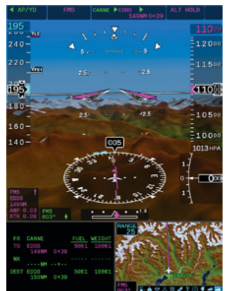
PFD with 360° HSI, Left Inset with Flight Plan Data, Right Inset with Map and SVS
