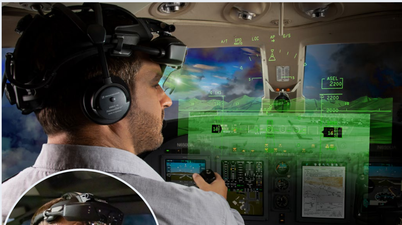
Above and inset, Universal Avionics has developed the Clearvision Enhanced Flight Vision System (EFVS), featuring a wearable display. Images: Universal
